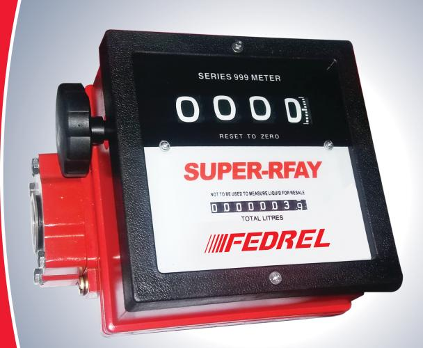
Mechanical volumetric flow-meter for private use, with mutating-disc type chamber for deliveries to 120 l/min. It can be installed for gravitational feeding, as well as for hand operated or electric transfer pumps with by-pass arrangement.
