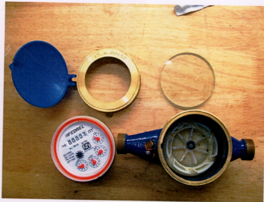
PLATE C: WATER METER AFTER COMPLETION OF IP X8 TESTS
