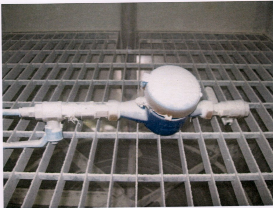
PLATE A: WATER METER AFTER COMPLETION OF IP 6X TEST
