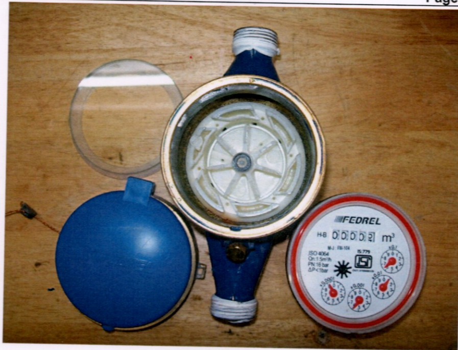
PLATE B: WATER METER AFTER COMPLETION OF IP 6X TEST
